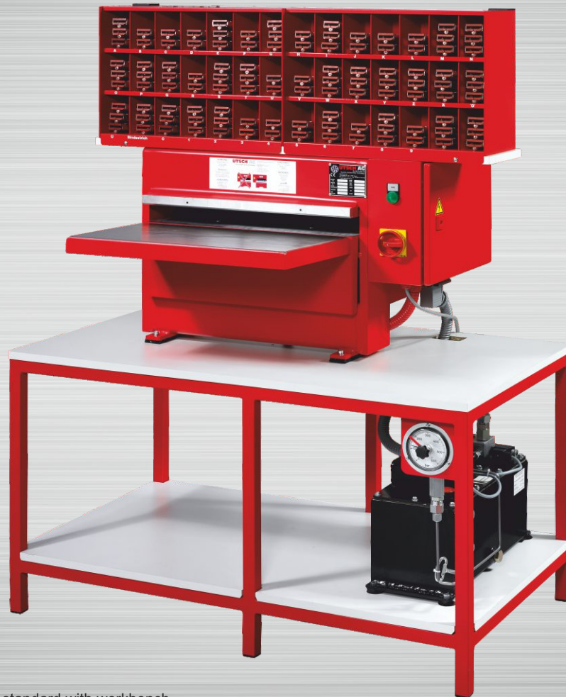
Embossing press comes as standard with workbench and optional with shelf for clapper dies as an accessory.
