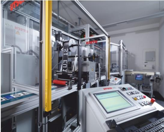
Depending on the degree of automation, an output of up to 400 pairs (800 plates) per hour can be realised with one operator only.
