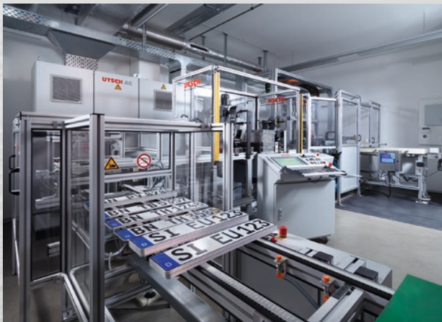
The Automatic Embossing Press for the computer-controlled, fully automatic manufacture of vehicle license plates in large quantities.
